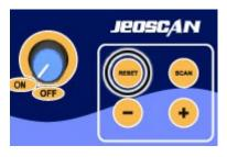
are eliminated. Resetting should not be done when the detector head is over the target! This will cause loss of depth, misinterpretation of received signal and the target become invisible to the device. Resetting procedure is carried out after the detector head is removed away from the target.
