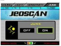
that turns from yellow to into green on "OFF" and press the "ACCEPT" button again. After this operation press "SETUP" button to switch to the previous mode. Following this step the device will filter worthless metals. To be able to detect worthless metals again this mode should be switched back to "ON" mode by repeating above mentioned operation.
